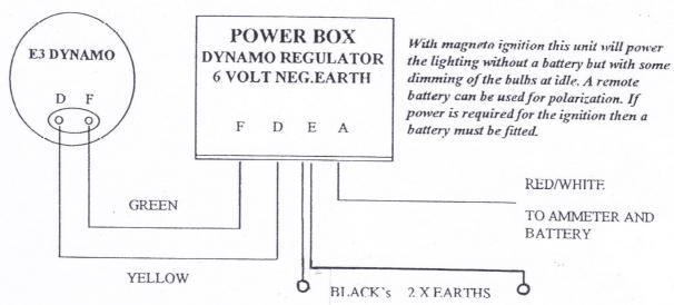
MOUNT IN ANY POSITION, THE LUCAS COVER CAN BE PUSHED OVER THE UNIT AND HELD WITH LOCKING WIRE OR CLEAR PLASTIC STRAP. THIS WILL GIVE AN ORIGINAL APPEARANCE WHEN REQUIRED
